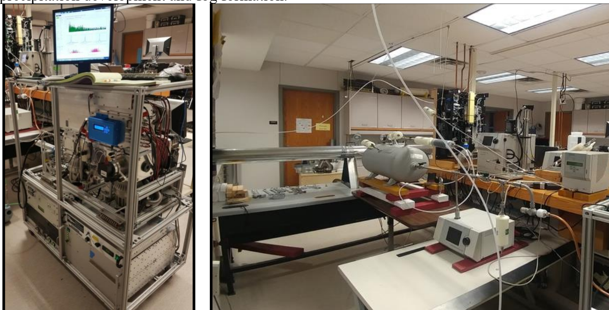
Figure 2: The left image shows the Aerosol Mass Spectrometer (HR-ToF-AMS) at the University of North Dakota's Clifford Hall 423, Instrumentation and Chemistry Laboratory during August 2020. The right image shows aerosol instruments own by the University of North Dakota (UND) and Weather Modification International (WMI) that sampled concurrently with the AMS. The aerosol instruments shown include (middle of the wood top bench) a Scanning Mobility Particle Spectrometer Particle (SMPS), which is required for AMS calibrations.
